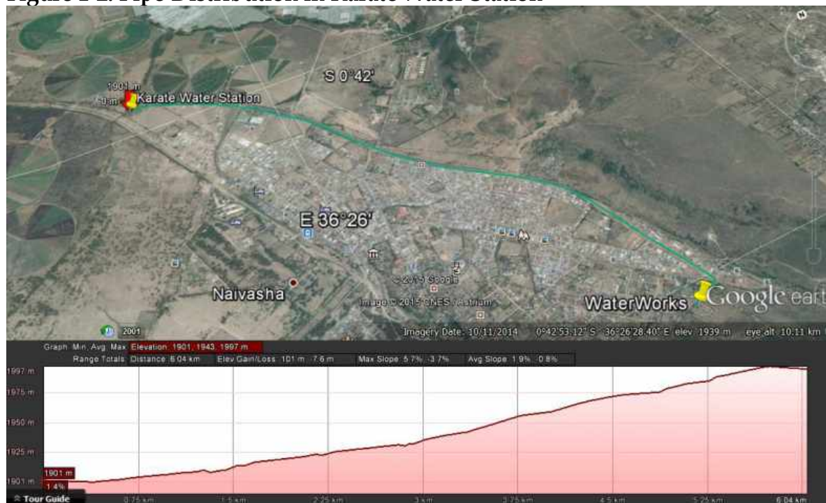
Figure 1-2: Pipe Distribution in Karate Water Station
